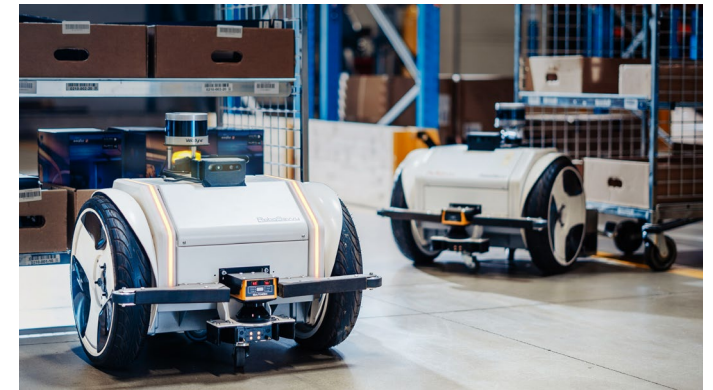
At our location in Greven-Reckenfeld, two Autonomous Mobile Robots help with the storing of small items.
